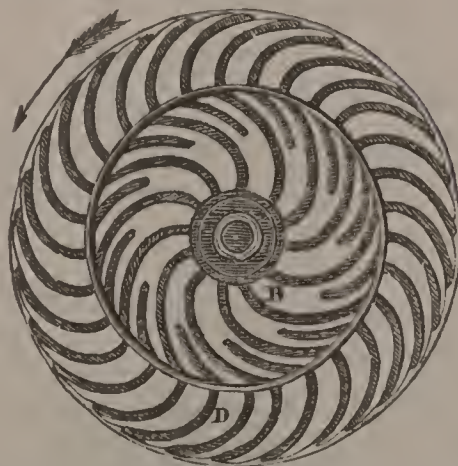
Turbine Wheel. B, curved partitions; D, working-wheel.
